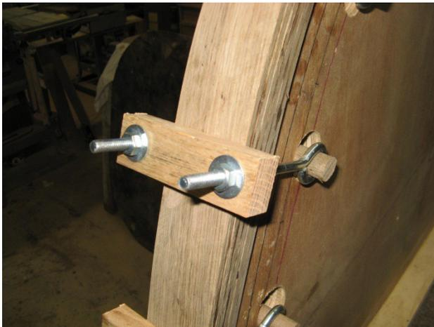
To make the stem I purchased a white oak board that measured 2x6x60 and ripped the oak into 17 1/8 strips. The white oak board cost \$37. As you may know, white oak bends extremely well but it needs to be soaked in water prior to bending. I then soaked 8 strips in water for 3 days
